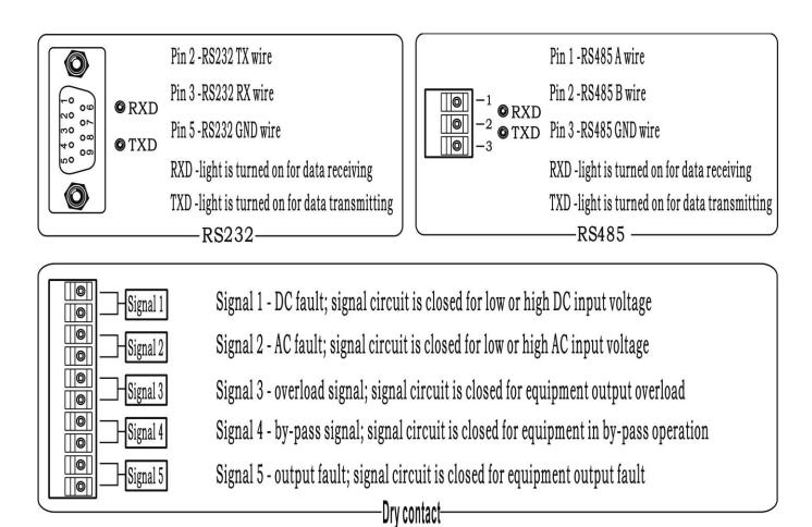
Note: the contact capacity of each group of the dry contacts shall not exceed 60 V 0.5A.
